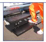
Flip Down Step Optional flip down second step bolts to standard rear step and is designed to help prisoners with leg shackles. Slam latch keeps it in stored position during vehicle operation KK-ST-FLIP
